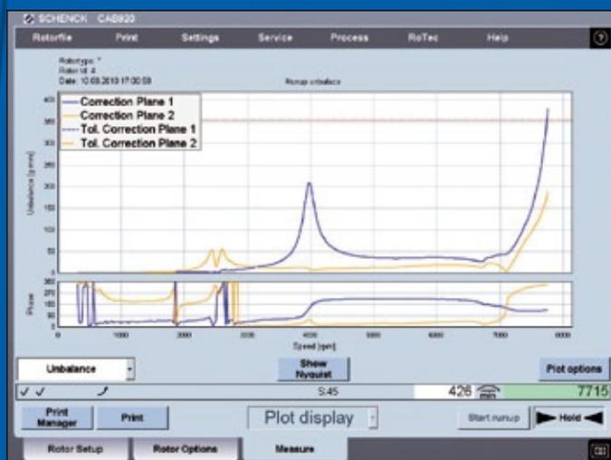
The unbalance effect of a flexible rotor can be measured during start-up displayed in a Nyquist diagram.
